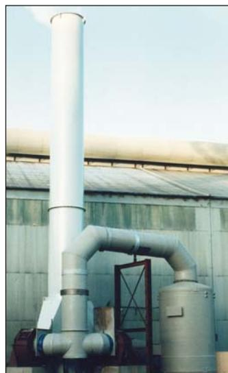
During operation, the gas to be cleaned flows vertically upward into the tray section through the sieve holes or capped risers, which can vary up to 1-inch diameter. Scrubbing liquid is introduced to the top tray where it flows in a horizontal cross flow direction to the gas rising over the tray's surface. The gas velocity through the tray openings, holds the liquid up on the tray and creates a froth layer where violent gas and liquid contact occurs to
