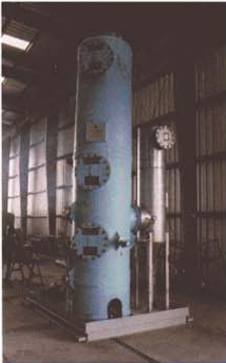
This ScrubPac™ is designed to quench and remove high temperature 1600°F hydrochloric acid gas emitted from a hazardous waste treatment reactor. Designed for completely automatic operation, the unit was engineered, manufactured, installed and operational in just 10 weeks.
