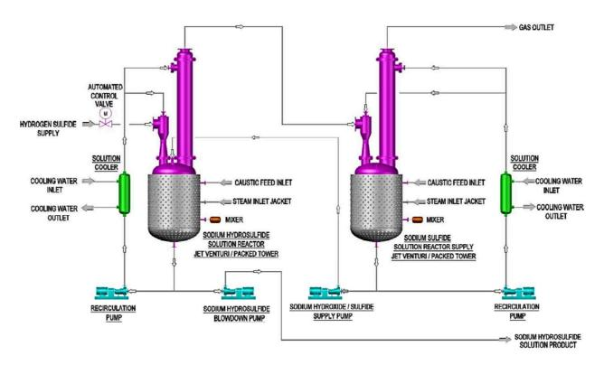
The standard system can be tailored to produce a large variety of NaHS solution concentrations ranging from 20% through 45%. The system can be configured with the logic to operate fully automated in either a batch or semi-batch continuous operation. Redundant instrumentation and transfer pumps adds to the systems overall excellent operational reliability.
